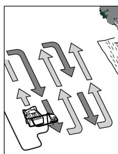
Place the ALR 900/AVR 1100 on the edge of the lawn, as close to the power point as possible. Work away from the power point.
