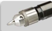
SM-74-7253P-03 with 1/2" Industrial keyed chuck
