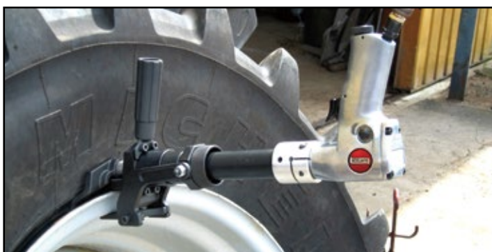
▲ Operation of Bead Breaker
