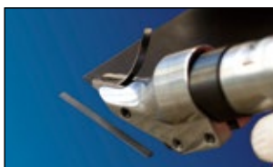
▲ Operation of Air Metal Shear
