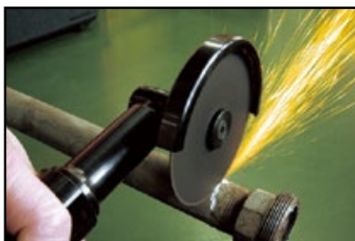
► Operation of Cut-Off Tool
