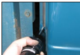
▲ Operation of Spot Drill
