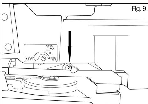
a growing oil stain then chain lubrication is working properly. If there are no oil stains on the ground, adjust the lubrication strength on the underside of the chain saw (Fig. 9)
