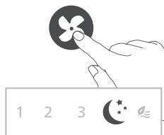
**Natural breeze mode (⾵):** Adjusts fan speeds up and down to mimic the natural movement of air and bring the refreshing feeling of an outdoor breeze into the room.
