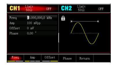
Press Freq soft key to set the frequency, use numerical keyboard to input 2 and then select the unit of parameter to kHz;
