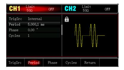
Press the corresponding soft key to set a parameter, to input numerical value and then select the unit.
