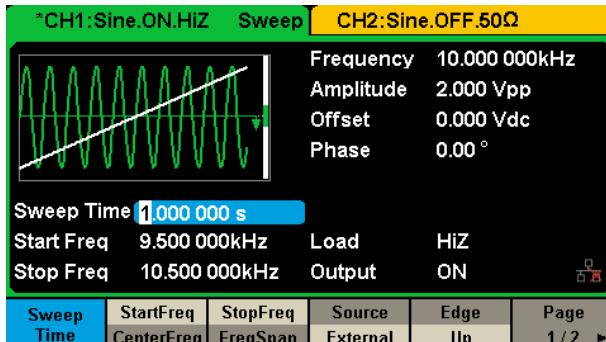
Two Sweep modes, "Linear" and "Log". Two Sweep directions, "Up" and "Down" and three Sweep sources, "Internal", "External" and "Manual".
