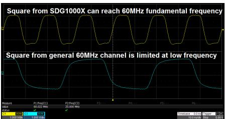
Benefitting from a special square-wave generating circuitry, the Square from the SDG1000X breaks the 60 MHz bandwidth barrier, reaching rise/fall times of less than 4.2 ns, and frequencies up to 60 MHz.
