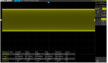
SDS1004X-U can measure all sampled data points up to 14 Mpts. This ensures the accuracy of measurements while the math co-processor decreases measurement time and increases ease-of-use.
