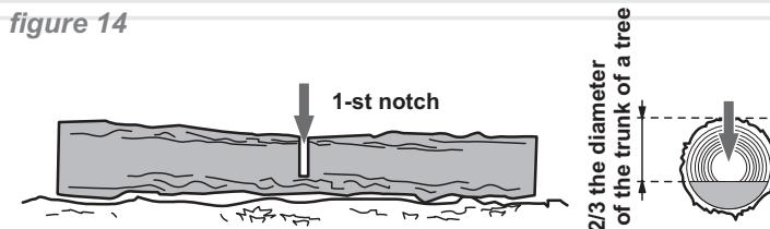
1. Make the first cut down to 2/3 the diameter of the trunk of a tree (see Figure 14).
