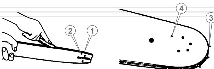
1. Remove dust and dirt from the gutter tires, oil holes and driven sprocket (see Figure 22).
