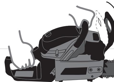
1. Place the chain saw on a flat surface. Make sure the tire chain is not touching any other object.
