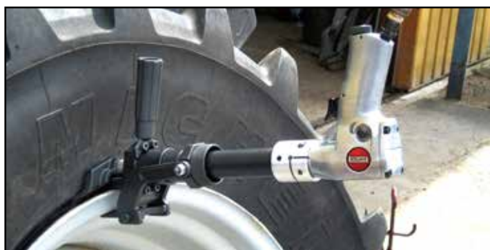
▲ Operation of Bead Breaker
