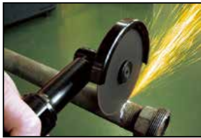
► Operation of Cut-Off Tool
