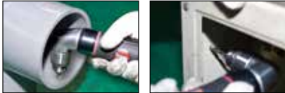
▲ Operation of 3/8" Reversible Angle Drill
