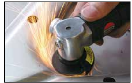
▲ Operation of Cutting Metal Plate
