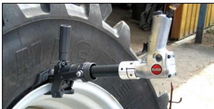
▲ Operation of Bead Breaker
