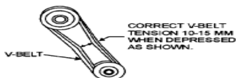
Figure 2. V-Belt Tension
